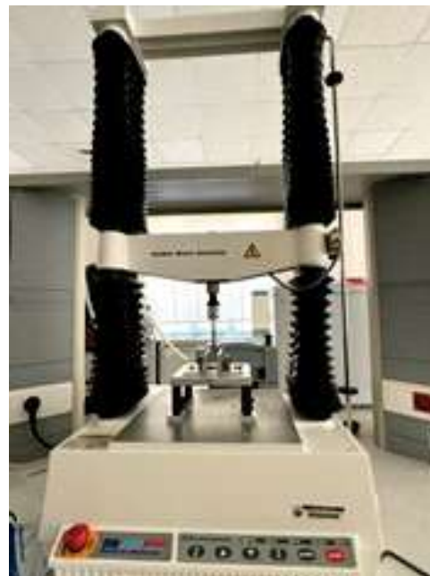
Fig 1: The Instron device used for the fracture test
