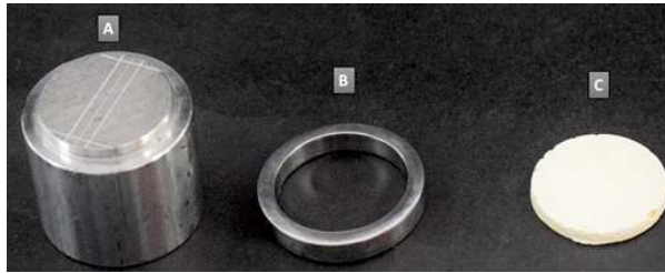
Fig 1: Different parts of Mould for Dimensional stability. *A; Block carrying the mould, *B: Ring, to confine mixed materials to mould, *C: Die used to press materials in mould
