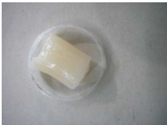
Figure - 2: Composite material inserted into the mould cavity
