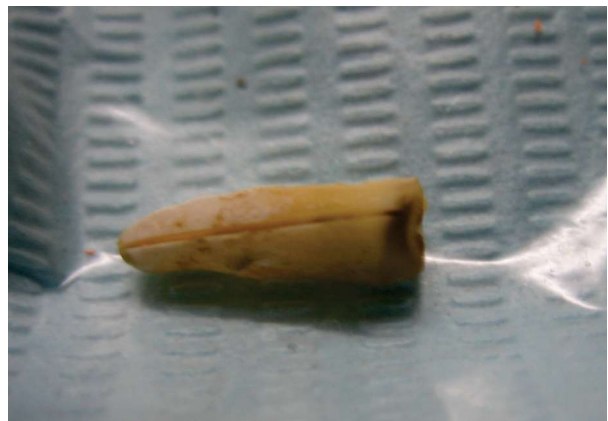
Fig 4: Grooves by diamond disc for splitting the specimen
